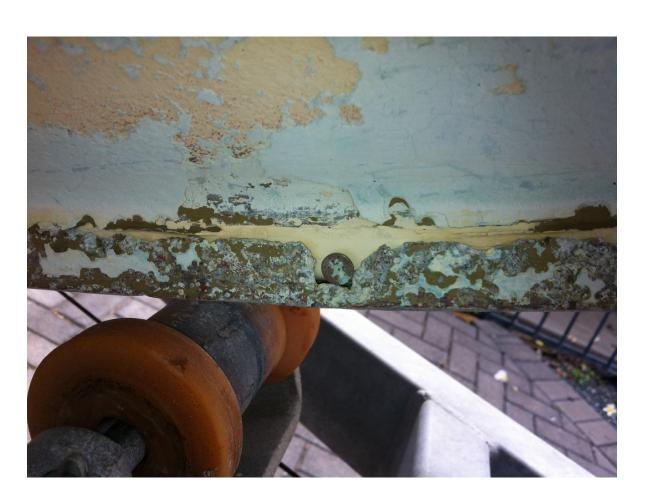
Caused by dissimilar metals in contact and in the same electrolyte with out anode protection.
