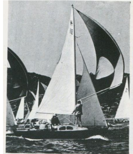
LOA, 6.7m. LWL, 5.5m. Beam, 2.2m. Draft, 1.15m. Sail area, 23.2sq m. Displacement, 1.6t. Ballast, 567kg. Boat in basic stage has glass-in berths and galley unit, without a rig. Sailaway stage has teak trim, bunk cushions and rigged with sails. No liferails or pulpits. Sailaway price around $6200. Builders: Sydney, NSW.
