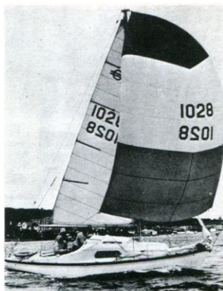
LOA, 7.2m. LWL, 5.5m. Beam, 2.3m. Draft, 1m. Displacement, 1.2t. Updated racer/cruiser. Fast and easy to sail. Basic accommodation, four berths, midship galley and WC. Sailaway price around $7400. Builders: Yachts, Hurstville, NSW.
