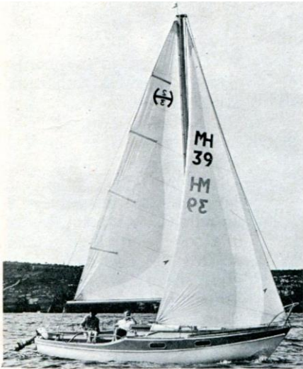
LOA, 7.2m. LWL, 5.7m. Beam, 2.25m. Draft, 1.25m. Sail area, 25sq m. Displacement, 1.7t. Ballast, 748kg. Excellent sitting head room and space below. Four berths in glass furniture, galley, WC and lighting. . . . race as a class in NSW and hold own state championships. Sailaway price approximately $7000. Builders: Boat Company, Sydney, NSW.
