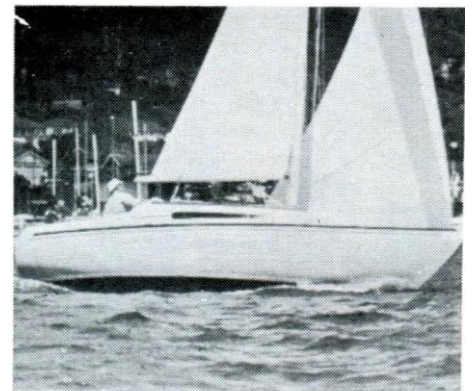
LOA, 7.5m. LWL, 6.2m. Beam, 2.7m. Draft, 1.4m. Displacement, 1.9t. Ballast, 771kg. Sail area, 23.5sq m. Practical all-purpose layout. Five berths, L-shaped galley to port, enclosed WC for'ard. With all berths aft of the mast step Triton 24 has a good layout to go to sea in. Sailaway price is around $10,200. Builders: Boat Company, Sydney, NSW.
