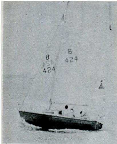
LOA, 7.2m. LWL, 5.5m. Beam, 2.5m. Draft, 1.5m. Displacement, 1200kg. Ballast, 500kg. Sail areas: Main, 9.7sq m. Genoa, 20sq m. Spinnaker, 40sq m. Designers: Akkerman and Kremer. Four berths, hinged chart table, two-burner stove, plastic sink, ice box, WC. Price around $5000. Builders: Melbourne, Victoria.
